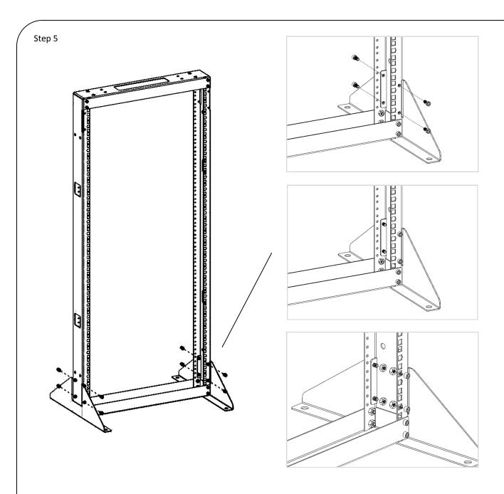
Assembly Tip: Hand tighten all bolts until the entire rack is assembled. Then go back and tighten them with the wrench.
